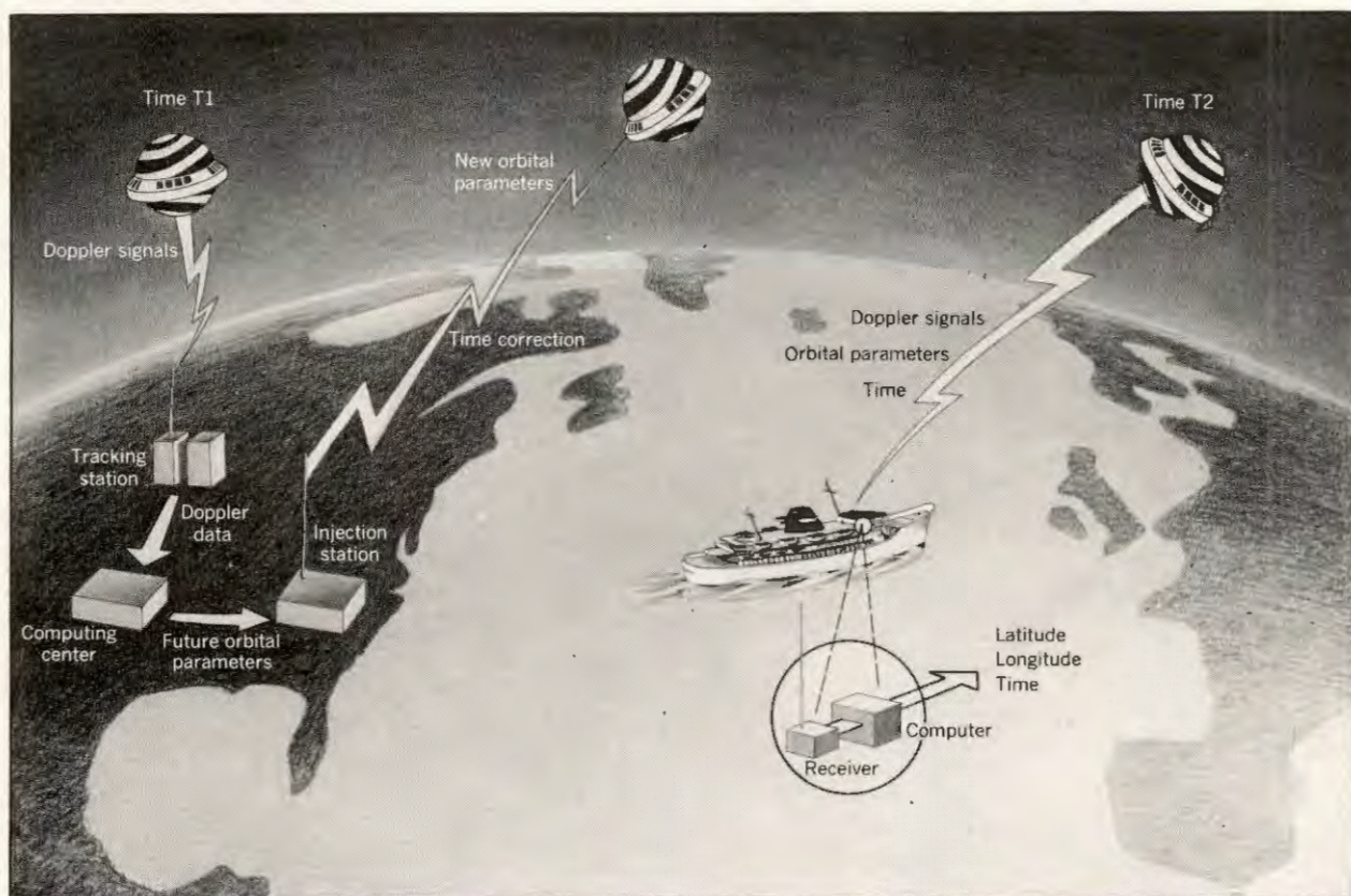
FIG. 15.--After launching of Transit I-B the satellite's Doppler signal is picked up by receiving station (time phase 1), which reduces it to digital form and transmits it to Central Computer Center at Applied Physics Laboratory of The Johns Hopkins University, Silver Spring, Md. Staff at computer center, using Doppler data, is able to predict future paths or orbital parameters of Transit I. These are relayed to injection station and then transmitted back to Transit I. Satellite stores the data and transmits it to earth intermittently (time phase 2). Ship navigators with receiver-computer equipment combine position information of satellite with current Doppler shift data to determine their position on earth.
